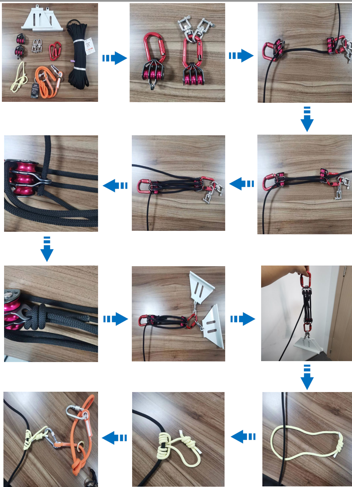
Figure 10 Assembly of pulley block
